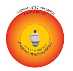
Each FIREBird device can detect fires as small as 6 ft by 6 ft  $(1/1000^{th} \text{ of an acre})$  up to 1000 feet distant.
