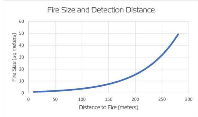
Figure 3: FIREBird Device Fire Detection Range vs Size
