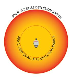
Each FIREBird device protects a 60-acre area. Detection of wildfires as small as 5 ft. by 5 ft. can be from as far away as 900 ft. Even smaller wildfires can be detected within 400 ft of the device.
